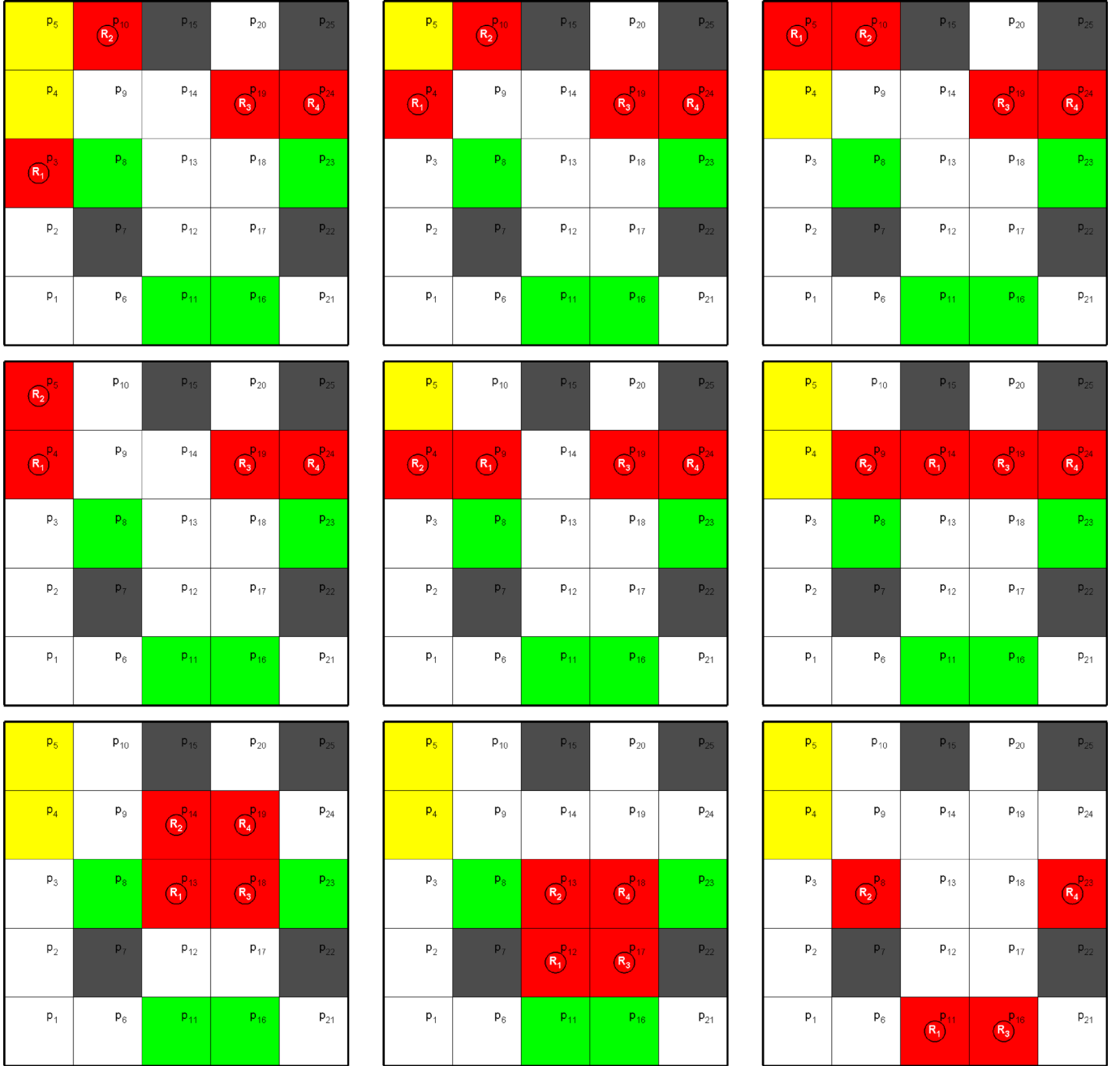
Fig. 5. Successive configurations of the team for the example in Section VI-A (the initial configuration is shown in Fig. 4). The regions occupied by the four agents are in red. Gray regions should be avoided, yellow regions should be visited, and green regions should be entered simultaneously.
