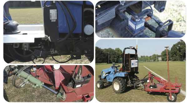
Fig. 1. On the top left side: the electromechanical valve, on the bottom left side: the electrohydraulic valve, on the top right side: the potentiometer, on the bottom right side: the articulated unmanned ground vehicle.
