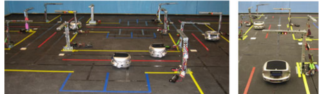
Fig. 1. Robotic urban-like environment. (Left) Khepera III car-like robots move autonomously on streets, while staying in their lanes, obeying traffic rules, and avoiding collisions. (Right) Car waiting at a traffic light.
