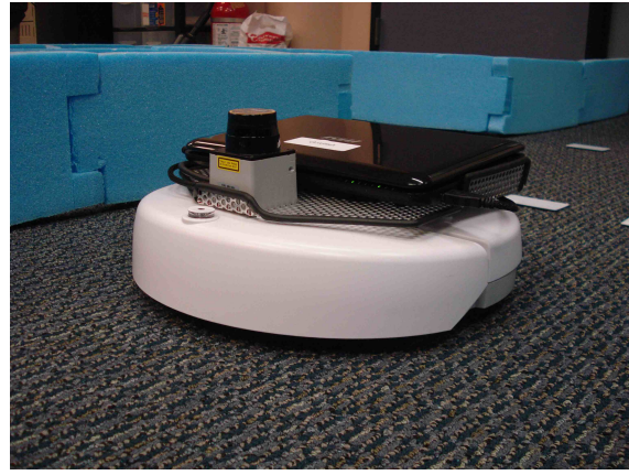
Fig. 1. Robotic InDoor Environment (RIDE). Left: An iCreate mobile platform equipped with a laptop, a laser range finder, and RFID reader moves autonomously through the corridors and intersection of an indoor-like environment, whose topology can be easily reconfigured by moving the foam walls. Right: A robot close-up.
