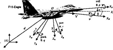
Figure 1: Body reference frames on an aircraft.
