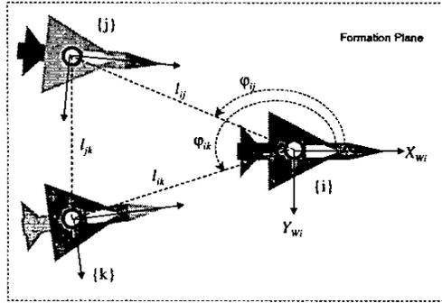
Figure 3: Three aircraft in a triangle formation.
