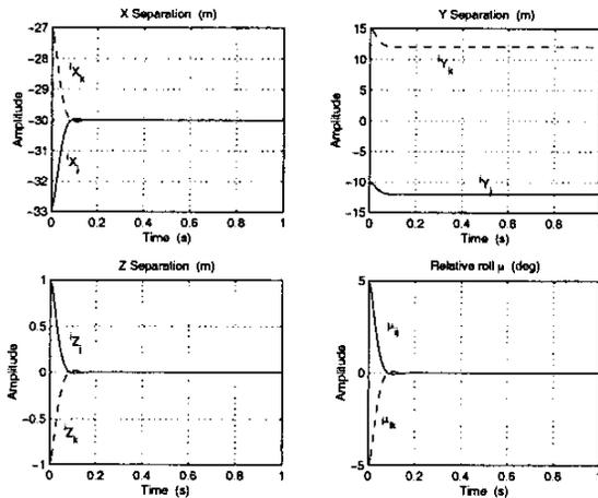
Figure 4: Controlled output variables of follower UAVs.
