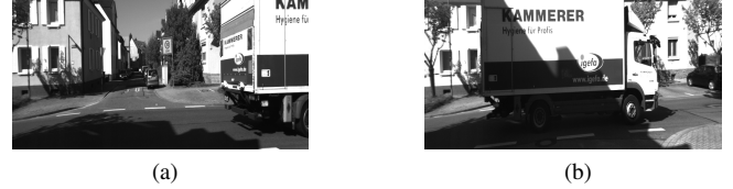
Fig. 5: Example in which the CNN cannot estimate the speed correctly due to the presence of an outlier (the truck crossing the street)
