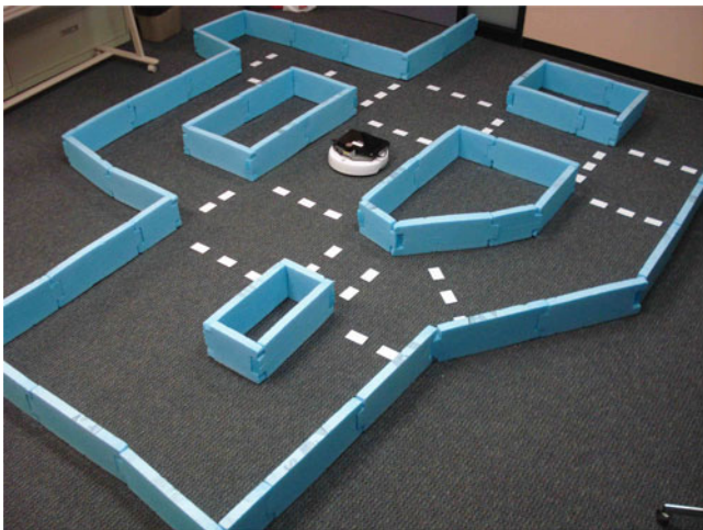
Fig. 1. Robotic indoor environment. (Left) iRobot Create mobile platform that is equipped with a laptop, a laser range finder, and RFID reader moves autonomously through the corridors and intersection of an indoor-like environment, whose topology can be easily reconfigured by moving the foam walls and (right) robot closeup.
