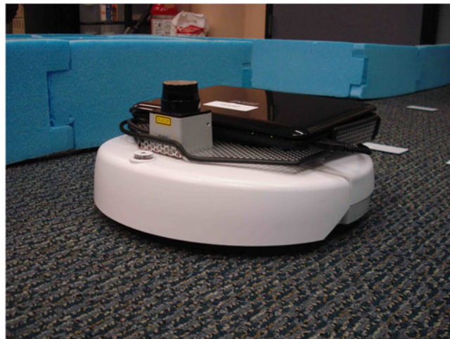
Fig. 1. Robotic indoor environment. (Left) iRobot Create mobile platform that is equipped with a laptop, a laser range finder, and RFID reader moves autonomously through the corridors and intersection of an indoor-like environment, whose topology can be easily reconfigured by moving the foam walls and (right) robot closeup.
