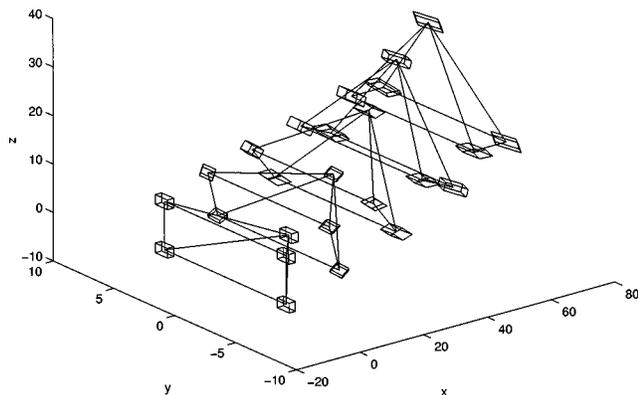
**Fig. 3 Optimal motion for five identical robots required to maintain a rigid formation**
