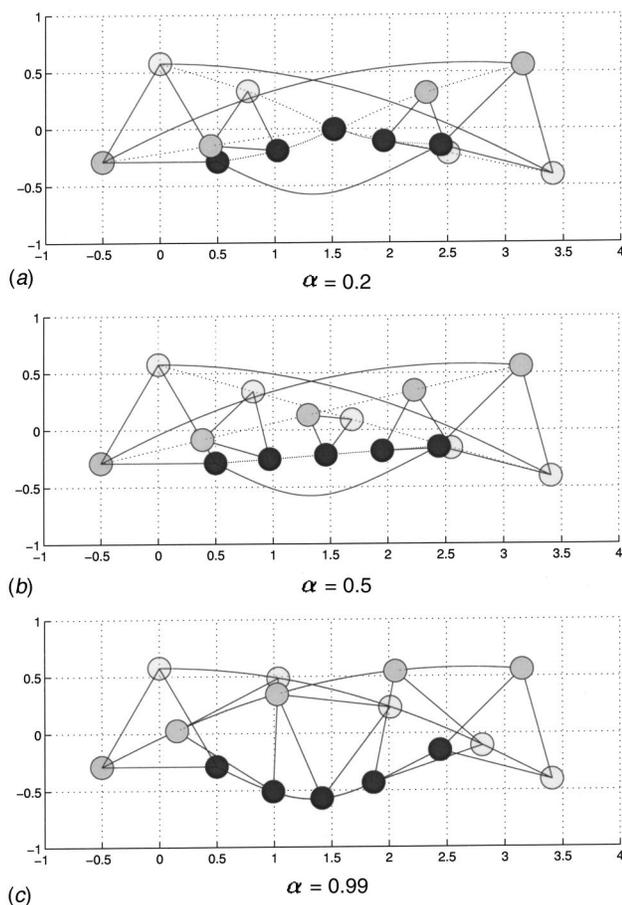
**Fig. 5 Three interpolating motions for a set of three planar robots as geodesics of a modified metric defined in the configuration space.**
