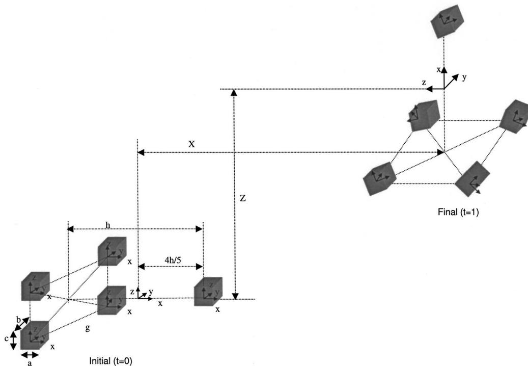
**Fig. 2** Geometry of the robots and of the virtual structure showing the initial and the final configurations. The relevant dimensions are chosen to be:  $a=c=2$ ,  $b=10$ ,  $h=20$ ,  $l=10$ ,  $X=20$ ,  $Z=20$ ,  $m=12$ .
