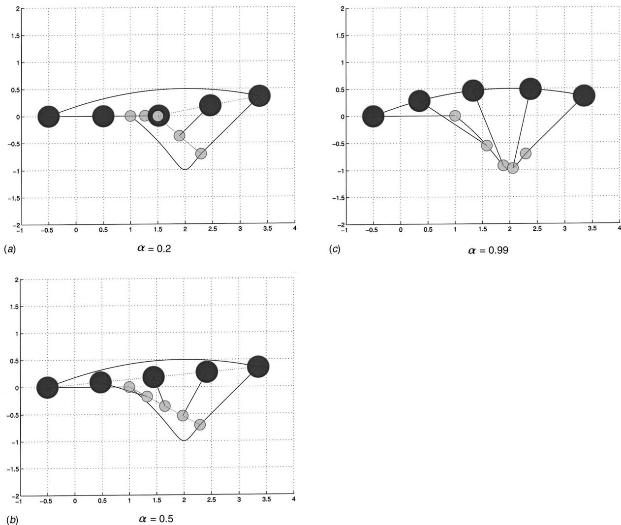
**Fig. 4 Three interpolating motions for a set of two planar robots as geodesics of a modified metric defined in the configuration space.**
