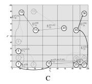
Fig. 2. A) Trajectories of the uncontrolled system go towards regions  $\mathcal{X}_{10}$  and  $\mathcal{X}_{27}$ . B) A simulated trajectory  $(x_1, \dots, x_{10})$  of the closed loop system. C) The control strategy used to generate the trajectory shown in B relied on 4 nondeterministic (dotted lines) and 5 deterministic (solid lines) transitions. States that were not visited by the trajectory but were targets of the nondeterministic transitions are also shown.
