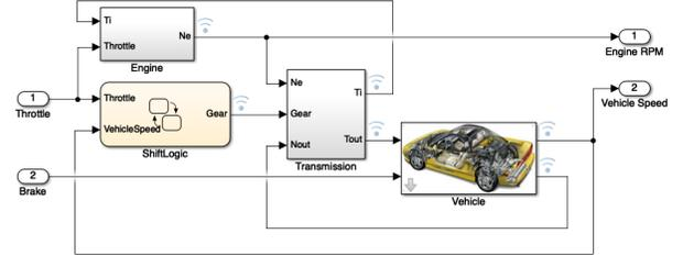
Fig. 3. The Simulink automatic transmission model diagram [21].
