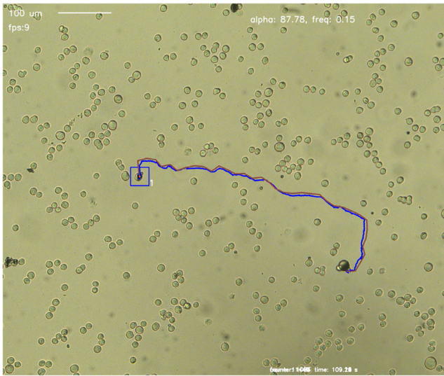
FIGURE 8 | Experimental results for a cellbot moving in an environment cluttered with other cells. The red curve represents the reference trajectory generated by the RRT* algorithm, while the blue curve shows the actual trajectory generated by our controller.
